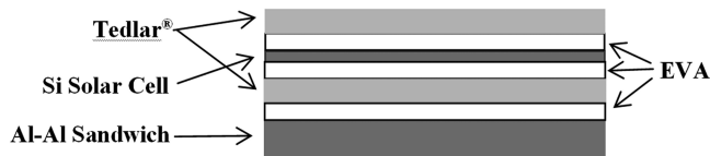
Fig. 1 Si terrestrial solar panel encapsulation and bonding on the structural substrate.
